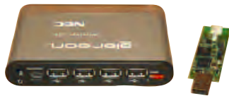
Wireless USB hub and dongle, with cover removed
